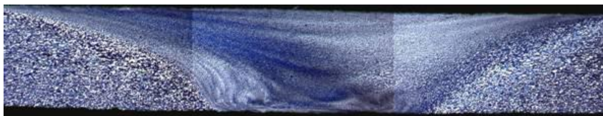
Fig. 5. Macrograph of the butt weld of AA7475-T7651 sheets of thickness of 1.27 mm.
