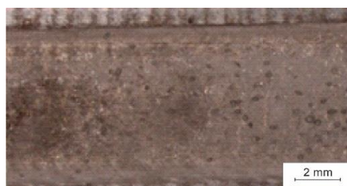
Fig. 7 Weld face after laser treatment with WC powder, MCMgAl9Zn1 alloy, scan rate: 0.5 m/min, laser power: 2.0 kW
