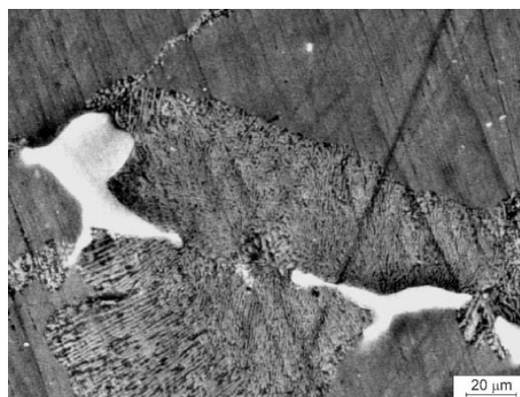
Fig. 2 Structure of the MCMgAl9Zn1 alloy after aging at the temperature of 190 C for 15 hours
