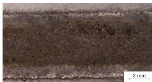
Fig. 8 Weld face after laser treatment with SiC powder, MCMgAl9Zn1 alloy, scan rate: 0.5 m/min, laser power: 2.2 kW
