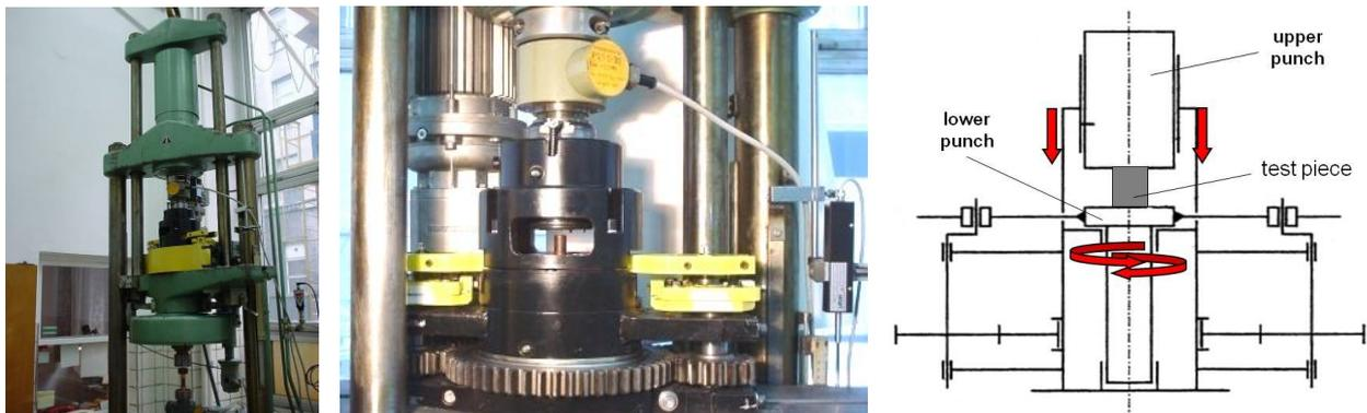
**Fig. 1** A device for compression with oscillatory torsion: as mounted in the material strength testing machine (left), a close-up view (center) and a schematic view (right)
