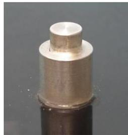
**Fig. 7** Nanostructured specimen of ECAE process prepared for RF process
