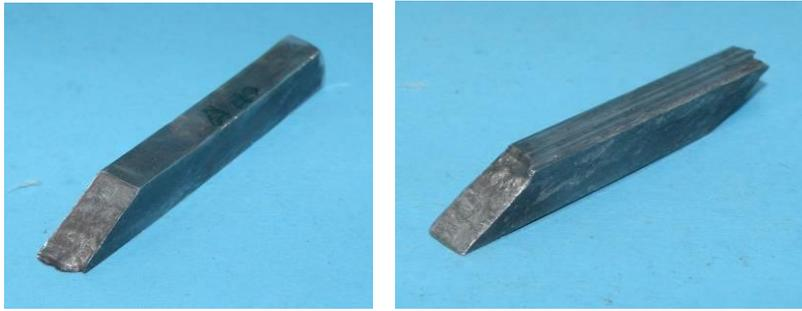
**Fig. 2** AIMg3 alloy specimen formed by ECAE technology
