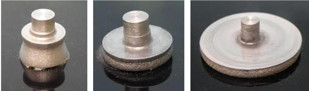
**Fig. 10** The phases of RF procedure – AlMg3 alloy – nanostructured
