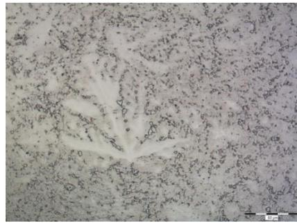
**Fig. 6** Microstructure of AZ80
