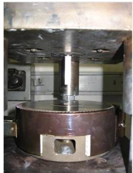
c) Detail of the forming tool with reheating sleeve
