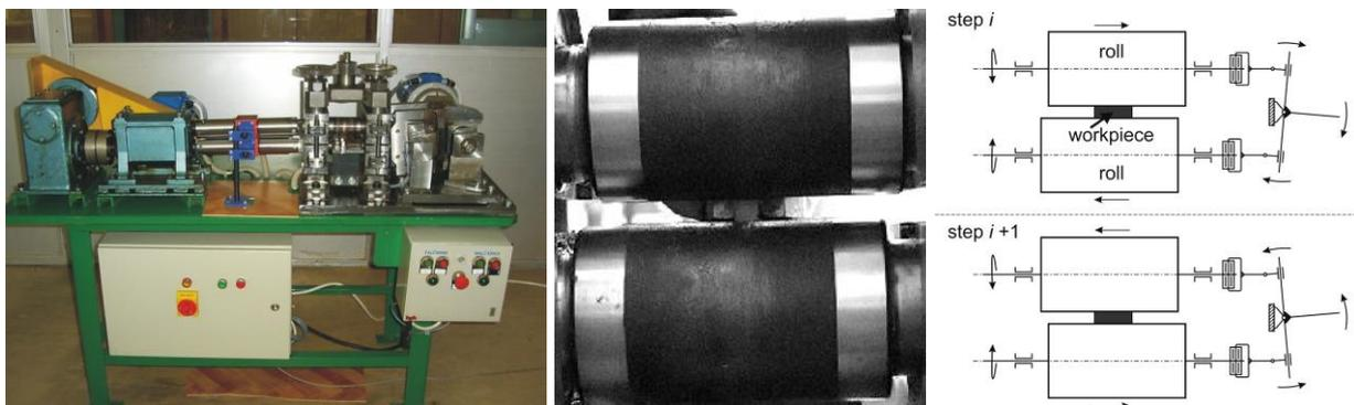
**Fig. 6** A laboratory stand for rolling with transverse rolls motion (left), a close-up view on the rolls and a workpiece during the test (center) and a schematic view (right)
